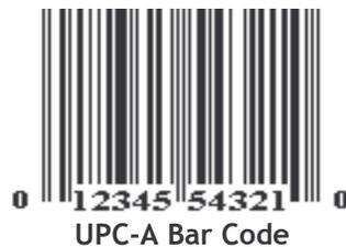
Bar codes are “read” by a device called a “reader” or “scanner”. These devices use reflected light off the bar code symbol to measure the widths of the bars and spaces.
